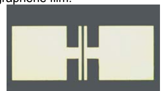
Fig.8. OM image of back-gated graphene FET.
